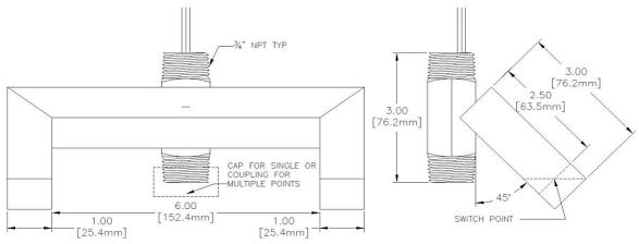
Repeatability: 2mm or better. Delay (on): 0.5 seconds Standard. Probe material: 316SS Standard. Actuation point: 3.0" Standard. cable Up to 50" available. Sensor Temperature: -20° to 150°C Sensor Pressure: 1000 PSIG 316LSS. Liquid viscosity : From 1 to 75,000 cps Process connection: ¾" NPT Standard Input options: 24VDC, 90 to 240VAC, Output Options: 10A DPDT Loop Power 4-16mA Push Button Demand Self-Test Field Select Fail-Safe Option
