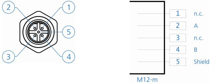
Figure 11 Connection diagram LDM301P Profibus-IN
