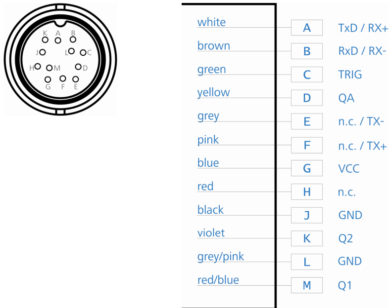
Figure 9 Connection drawing of the main connector
