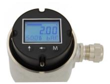
Unscrew the cover to get access to the push buttons of the display. The display can be turned max. 180° to put it in the desired position for reading. The complete display unit can be taken out to be able to adjust the transmitter. Be careful when taking out the display as the length of the wiring is limited. Please ensure that the cover is fastened properly after adjusting the display to ensure the sealing of the housing.
