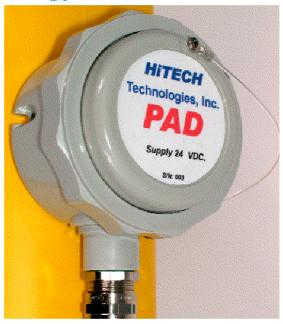
The **HITECH PAD** Through-the-Wall sensor is a presence-absence switch that detects the presence of materials based on a frequency shift of the sonic signal it applies though the media.
