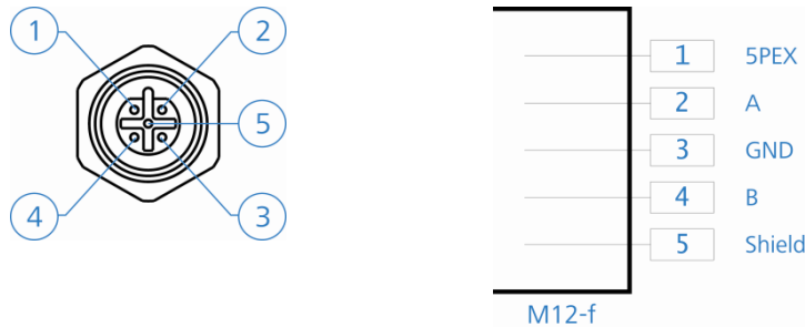
Figure 11 : Connection diagram LDM301P Profibus-OUT
