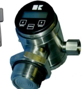
The Series 2000 SMART Pressure - Level Transmitters are solid state intelligent transmitters that provide a standard analog output (4 -20 mA), a local digital display and optional HART protocol or PROFIBUS-PA interfaces.
