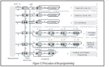
For entering programming mode: step **A** for 2 s For quitting programming mode: step **B** Programming mode entered: is indicated by blinking red and going off yellow and green LED s. While in programming mode (with red LED blinking) every step **A** will change the Menu Points. The six different Menu Points are indicated by combination of states of yellow and green LEDs.
