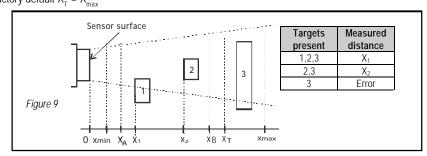
Far-end blocking will prevent evaluation of echoes coming behind  $X_T$ . Should for any reason (unstable echo, intensive movement of air) the echo be lost, the object behind  $X_T$  will not be taken into consideration but lack of the valid echo will immediately trigger error indication.
