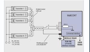
Wiring of Combined Systems (containing both 2- & 4-wire transmitters)
