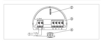
Electronics and terminal compartment, single chamber housing
