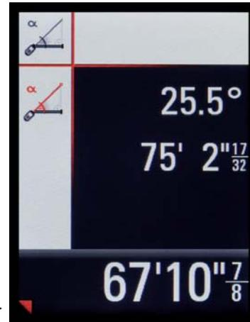
This little red triangle means there is a second screen with additional values. Press and hold the tilt button to access the second screen. Press and hold again to return to the first screen.
