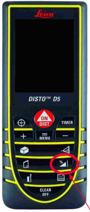
Press 4x on the D5 and 2x on the D8 to access the function. This symbol will appear in the top left corner
