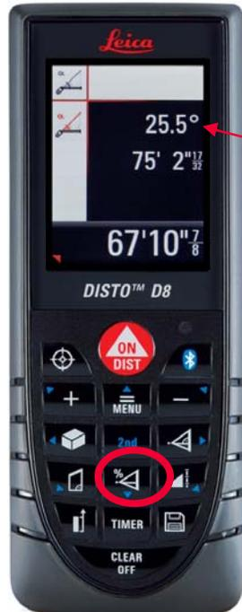
By accessing the menu, you can set the tilt sensor to display in percent, degrees, or inches/feet (rise over run). You can also activate the degree sensor to be active all the time in the point finder display at the top right hand corner.
